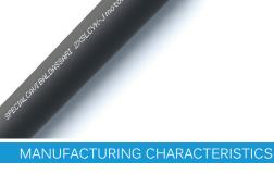
Conductor: Flexible bare copper, class 5 Insulation: **XLPE** compound Stranding: Cores stranded in concentric layers Wrapping and protection: Overall polyester tape Shield: 1st shield: Overall aluminium/polyester tape 2nd shield: Overall tinned copper braid Outer sheath: Flame retardant PVC compound Colours: Cores identification: Brown + Black + Grey + 3 x Green/Yellow Outer sheath colour: Black (based on RAL 9005)
